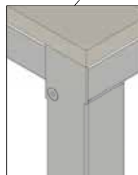
PIVOT ON WHICH THE LEGS ROTATE TO FOLD UNDER THE DESK TOP
